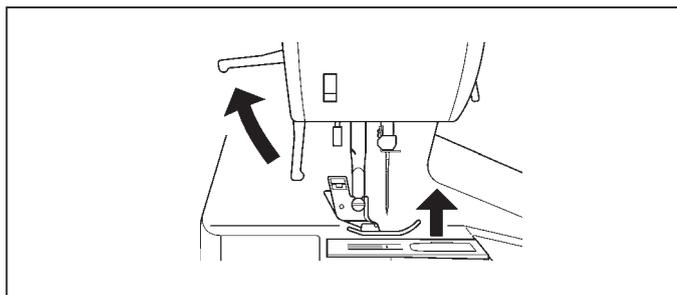
B. Turn the hand wheel toward you until the needle is in its highest position and the thread take-up is visible.
