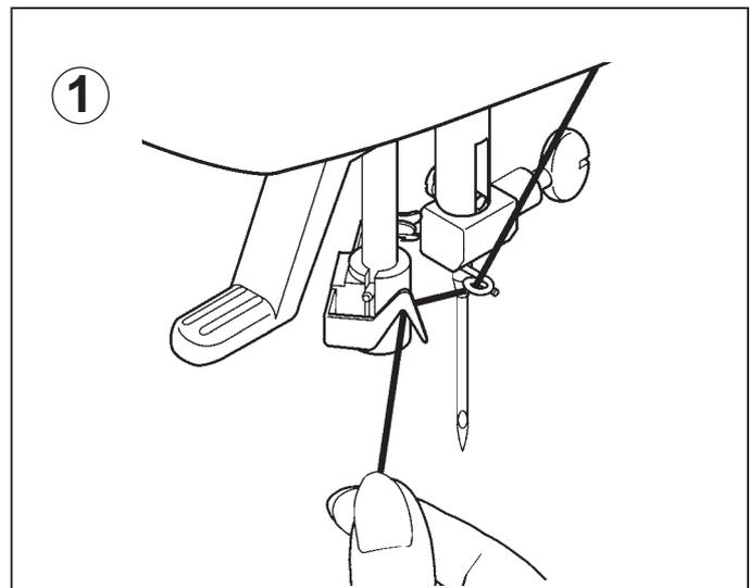
2. Pull down threader lever until the hooked end passes through the needle eye. Guide thread into hooked end and pull it upward.
