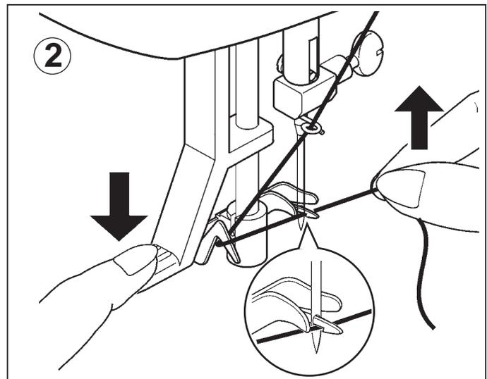
3. Release the threader lever and thread simultaneously, and needle will be threaded automatically.
